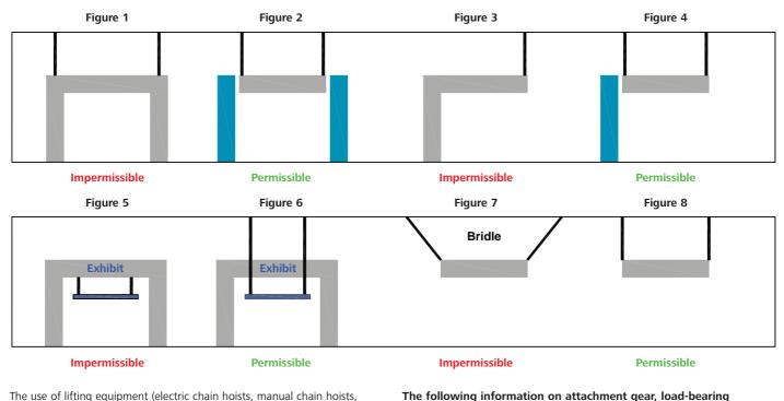
The use of lifting equipment (electric chain hoists, manual chain hoists, sling hoists) is only possible in halls 3A, 4A, 7A, 11 and NCC Ost and must be agreed with NürnbergMesse/Facility & Event Services.
