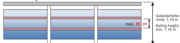
**Note:** In this case (with horizontal bars), the type of glass used can meet the specifications of Part 9 - Table A, glazing not intended to protect against falls. In the case of accident prevention balustrades in areas that are freely accessible to the **general trade fair public**, only vertical cross-bars should be used at the above-mentioned distance in front of the glass sheets, so as to prevent people (particularly children) from climbing over the balustrades.
