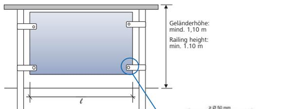
**Note:** If the types of glass and the dimensions listed in Table B are used, only static structural proof calculations are required for all point-fixed variants sided or 4-sided).
