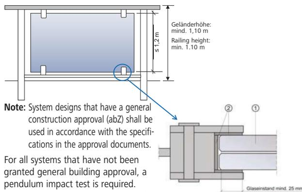
**Note:** System designs that have a general construction approval (abZ) shall be used in accordance with the specifications in the approval documents.
