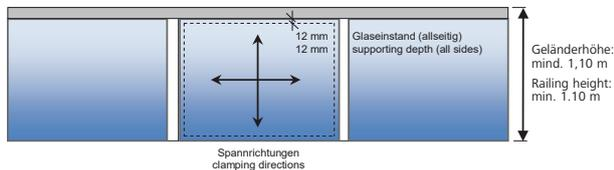
**Note:** If the types of glass and the dimensions listed in Table B are used, only static structural proof calculations are required.
