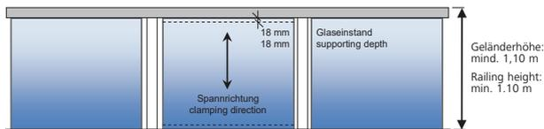
**Note:** If the types of glass and the dimensions listed in Table B are used, only static structural proof calculations are required.
