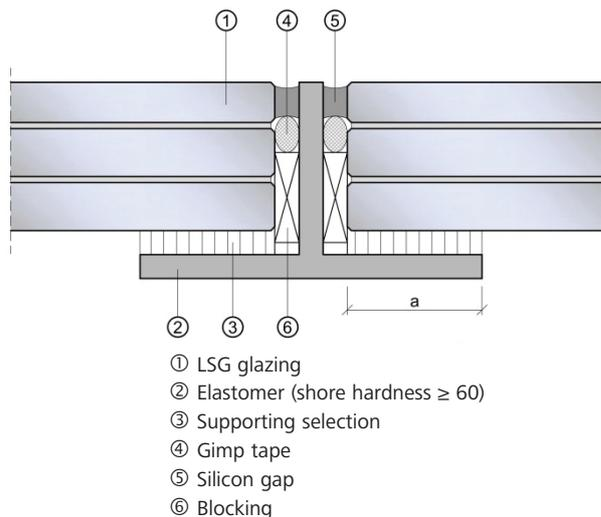
**Figure 2: Supporting surface depth a (glass insertion depth)**
