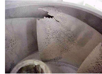
Pressure peaks of imploding bubbles lead to material erosion
