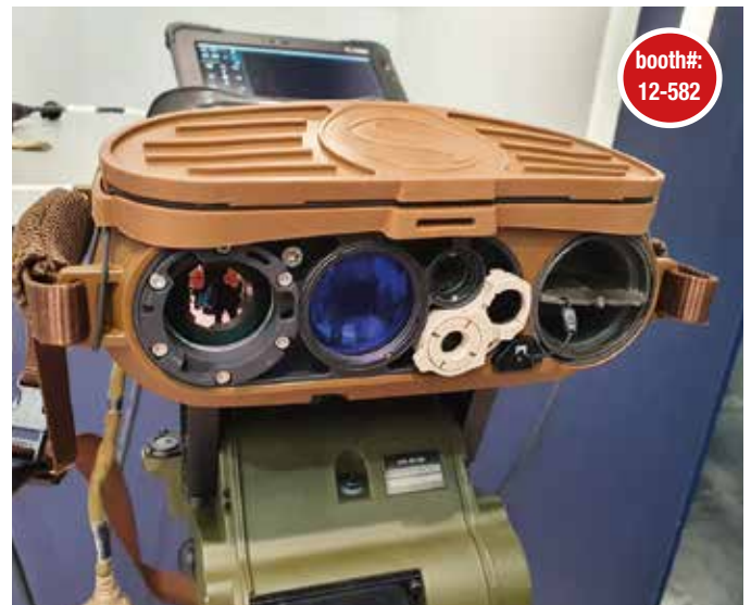
SAFRAN'S JIM Compact binocular weighs less than 2,000 grams, including batteries. (Stefan Nitschke)
