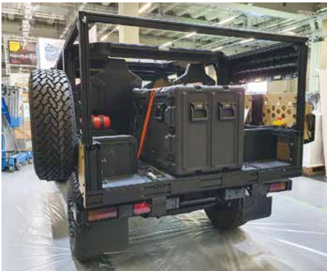
ENOK AB (airborne), designed with modern special forces in mind, features a GVW of 4,800kg, of which 2,000kg is payload. (Stefan Nitschke)
