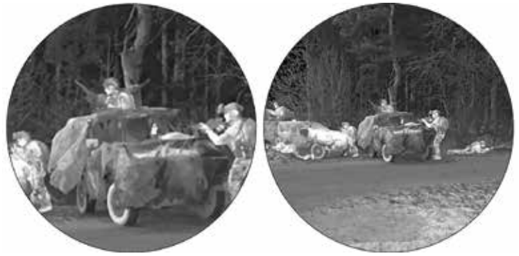
Comparison of conventional attachment (left, 36mm focal length) and PumIR-6M.5, at the same range but offering a much wider angle of view and improved sharpness. (Andres Industries)
