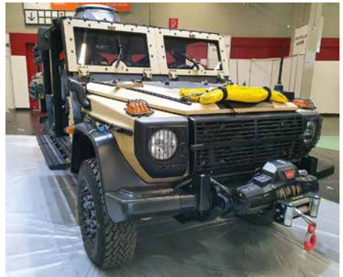
ENOK AB (airborne), designed with modern special forces in mind, features a GVW of 4,800kg, of which 2,000kg is payload. (Stefan Nitschke)
