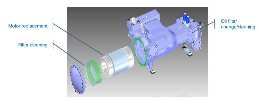
All maintenance operations can be done without removing the compressor
