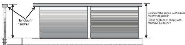
**Note:** If LSG made of 10 mm TSG + 1.52 mm PVB/SGP + 10 mm TSG or of 10 mm HSG + 1.52 mm PVB/SGP + 10 mm HSG in the dimensions as stated in Table B is used, only static structural proof calculations are required.
