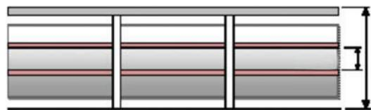
The type of glass used shall be selected from Table A, glazing not intended to protect against falls. The spacing between horizontal bars should not exceed approx. 35 cm.
