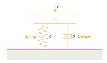
$$f_0 = \frac{1}{2 \cdot \pi} \sqrt{\frac{c_{dyn}}{m}} = \frac{1}{2 \cdot \pi} \sqrt{\frac{E \cdot A}{m \cdot d}} [Hz]$$
