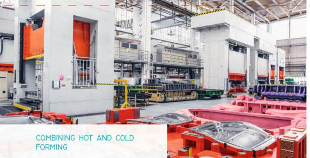
The Spanish forming specialist Gestamp presents a hinge column produced using the "Ges-Multistep" manufacturing process. The process combines cold and hot forming of sheet metal parts made of zinc-coated boron steel. A high-speed process that provides better corrosion protection even for complex geometries. To be seen during the Guided Tours and at a presentation in the AEE Congress. (Booth 12-328)
