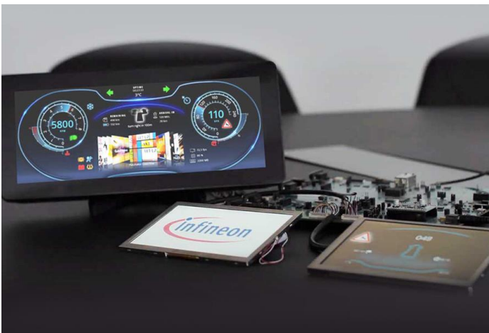
Image 2: Full virtual dashboard and dual Head-up display created with Candra CGI Studio on Infineon Traveo II
