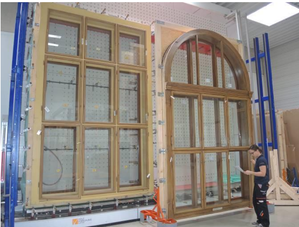
Caption: Historical windows being tested by Holzforschung Austria.
